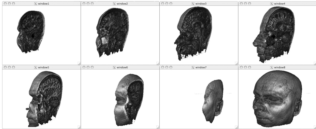
Figure 3.3: Sort-last parallel rendering of a large volume data set divided uniformly into slabs. Lower-right window shows final destination channel with back-to-front \alpha -blended slab images.
